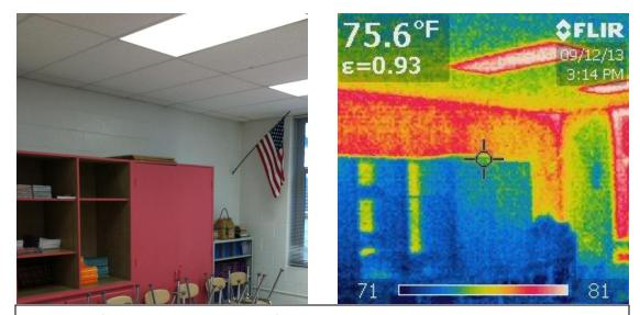
IR Photo of Room 31 showing heat infiltration along the back wall behind cabinets and at window near the Unit Ventilator. Wall behind the cabinets is a West facing wall and the IR image was captured at approximately 4:00PM.
