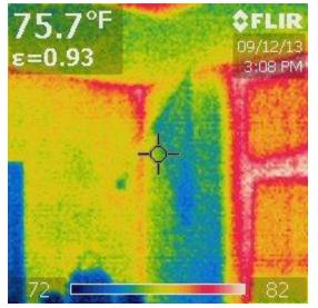
IR Photo of exterior wall and window in Room 31. IR Image indicates heat infiltration at window frame and corner of wall.
