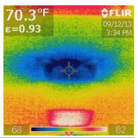
Supply air diffuser from Hallway Fan-Coil unit. IR Photo shows that the hallway unit is currently supplying 68 deg F air. No evidence of condensation at the time of the audit.
