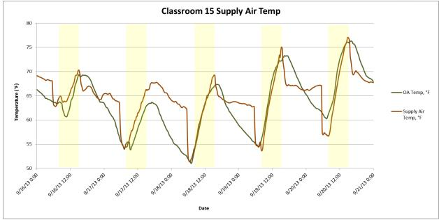
The above graph represents the supply air temperature (red line) discharging from the unit ventilator within Classroom 15. Supply air temperatures were high and out of the range needed to properly condition the space. However, the chiller was only operating on Thursday and Friday of the week. It appears that the chiller operation does not have an impact on the supply air temperature within the room indicating problems with the controls.
