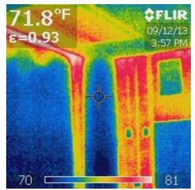
IR Photo of south wall in Room 11. Shows heat infiltration along south wall and around window frame. Negative air pressure within the building appears to be drawing air through cracks in the exterior wall and around the window frames.
