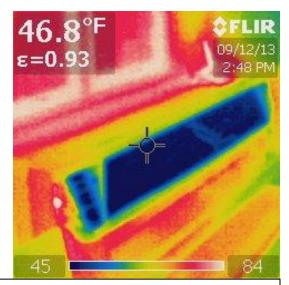
IR Photo of Room 33 Unit Ventilator interior showing cooling coil, unit interior and classroom window in background. The IR photo indicates heat infiltration inside the unit ventilator and around the window frame.
