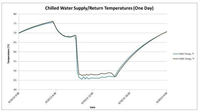
The above graph provides a summary of the chilled water supply & return temperature for a one day period. The chiller operated for only two days during the data logging time period. A  $2^{\circ}F$  temperature differential indicates only a small cooling load on the chiller.
