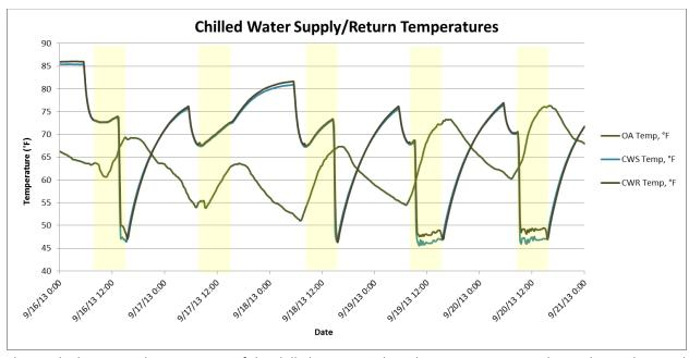
The graph above provides a summary of the chilled water supply and return temperature during the week. Based on the graph, the chiller was operated on Monday for a short time period and all occupied hours on Thursday and Friday. The chilled water supply temperature appears to be maintained at 46 to 47 deg F with little load on the chiller plant on Thursday and Friday.
