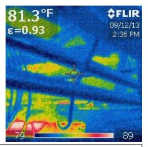
IR Photo above Room 33 ceiling tiles. Minimal heat loss through roof indicated.
