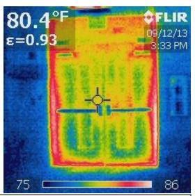
Exterior door in middle classroom wing hallway. IR Photo shows higher temperature around the door edges indicating air infiltration through the door edges.
