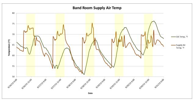
The above graph represents the supply air temperature (red line) discharging from the unit ventilator within the Band Room. The supply air temperature dropped during the night time hours indicating that the Trane unit remained operational throughout the unoccupied time periods or there was a large amount of air leakage through the Trane unit ventilator permitting outside air to cross over the data logger while the unit was off.
