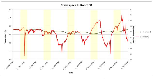
The abandoned steam tunnels are located under most classrooms in each of the classroom wings. The tunnels consist of block walls with dirt floors. One tunnel was checked during the site review and found to be very damp with a musty smell. The above graph provides a summary of the temperature and humidity in the tunnel crawl space during the week. As can be seen in the graph, there were periods when the relative humidity reached 93 to 96% RH while the temperature maintained a consistent 68 deg F.
