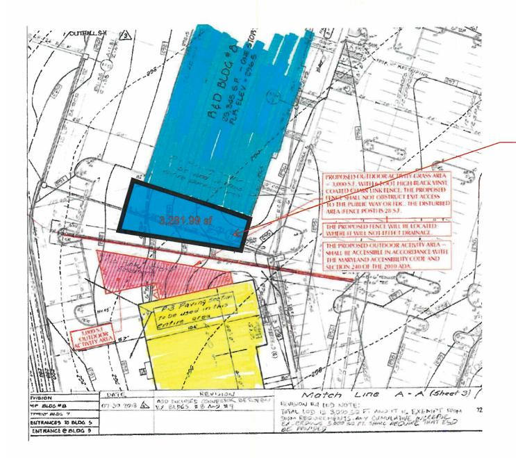
Make sure the fence foundation is not overlapping with 6" TAP and RCP
