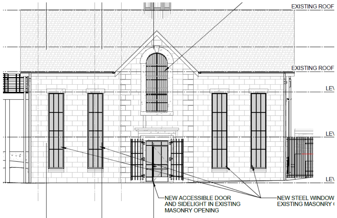
Figure 45 - Elevation showing restored window and door openings.
